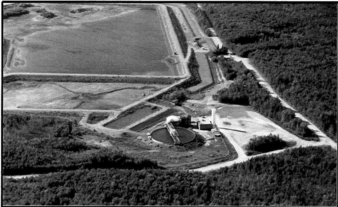
Water management, large open pit. Example of water management system with a collection pond in which pH is buffered (upper left) before being processed through an active water treatment facility (lower center). At east edge of the Brunswick No. 12 mine complex (see previous map), Bathurst, New Brunswick.
